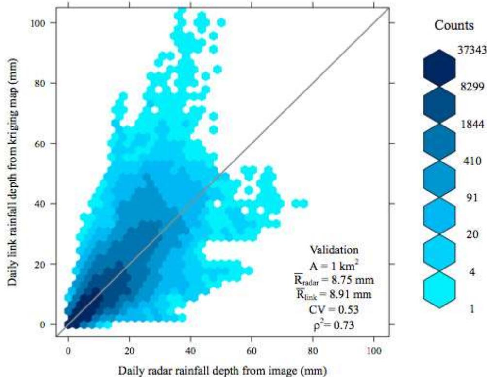
Validation of cell link rainfall estimates against corresponding radar rainfall estimates -- daily rainfall depths for each radar pixel of 1 km<sup>2</sup>. Only those rainfall depths have been used where link and/or radar have measured >0.1 mm. Gray line is y = x line; R = average rainfall depth at the radar pixel, CV = coefficient of variation, and  $\rho^2$  = correlation coefficient. Overeem et al. (2013).
