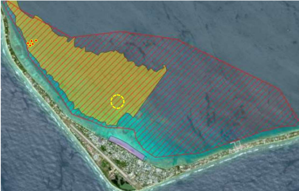
Figure 10: The olive-coloured zone is the established sediment resource area containing an estimated 24,000,000 m 3 of material which can be safely utilised (Smith, 1995). The larger red cross hatched zone is the area identified by Kaly and Peacock-Taylor (2014) as the “the zone of dead coral and eutrophication”. The yellow circle approximates the area which would be dredged to a depth of 3.5m to supply 350,000m 3 . The red/yellow dots are the (JP#) sample points detailed in Table 7 (Source: UNDP, 2019 and Hall, 2018).
