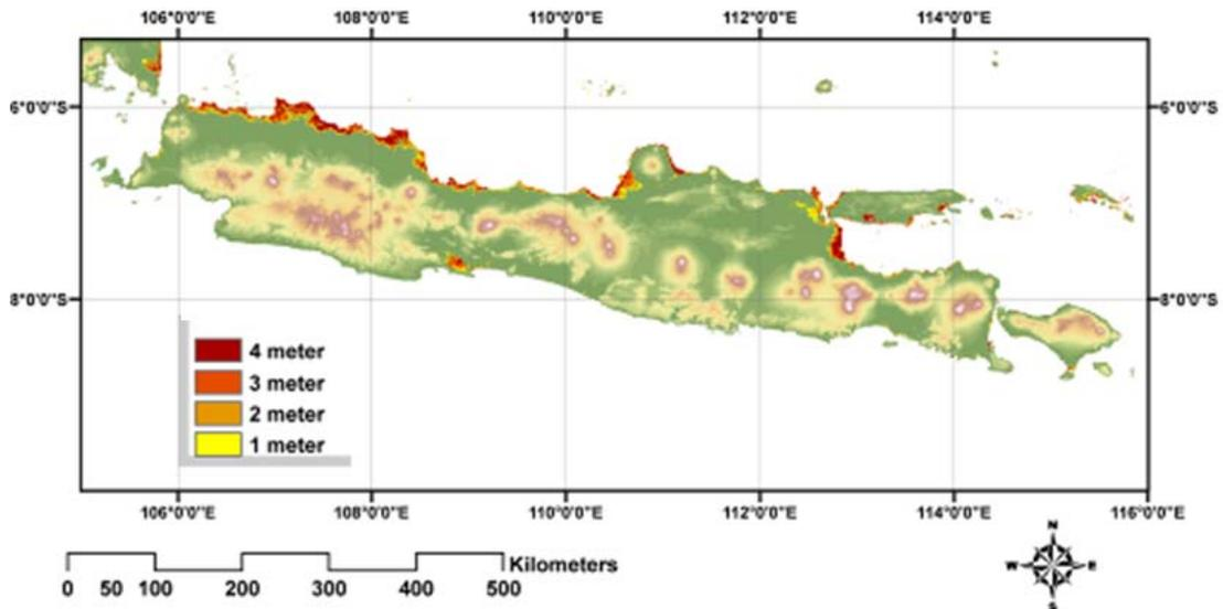
Figure 8 Simulation of Coastal Inundation in Java-Madura-Bali
