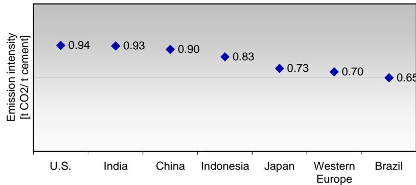
Figure 19 Examples of Emission Intensity in Cement Production
