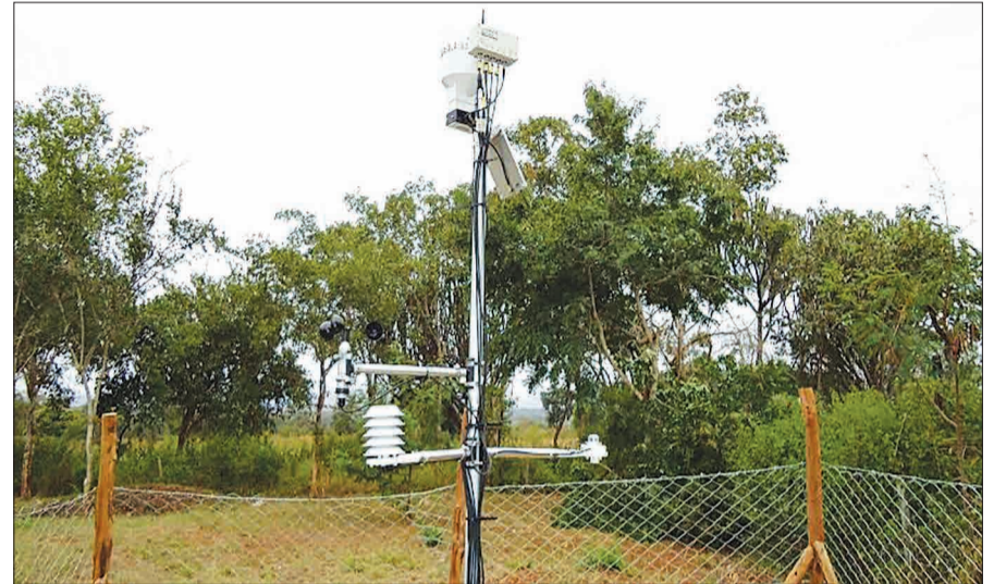
A modern weather station that has been installed by the GEF/UNDP-supported project on Strengthening Climate Information and Early Warning Systems (SCIEWS).
