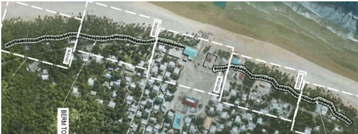
**Figure 76; Proposed alignment of the Berm Top Barrier concept design and footprint on Nanumaga.**
