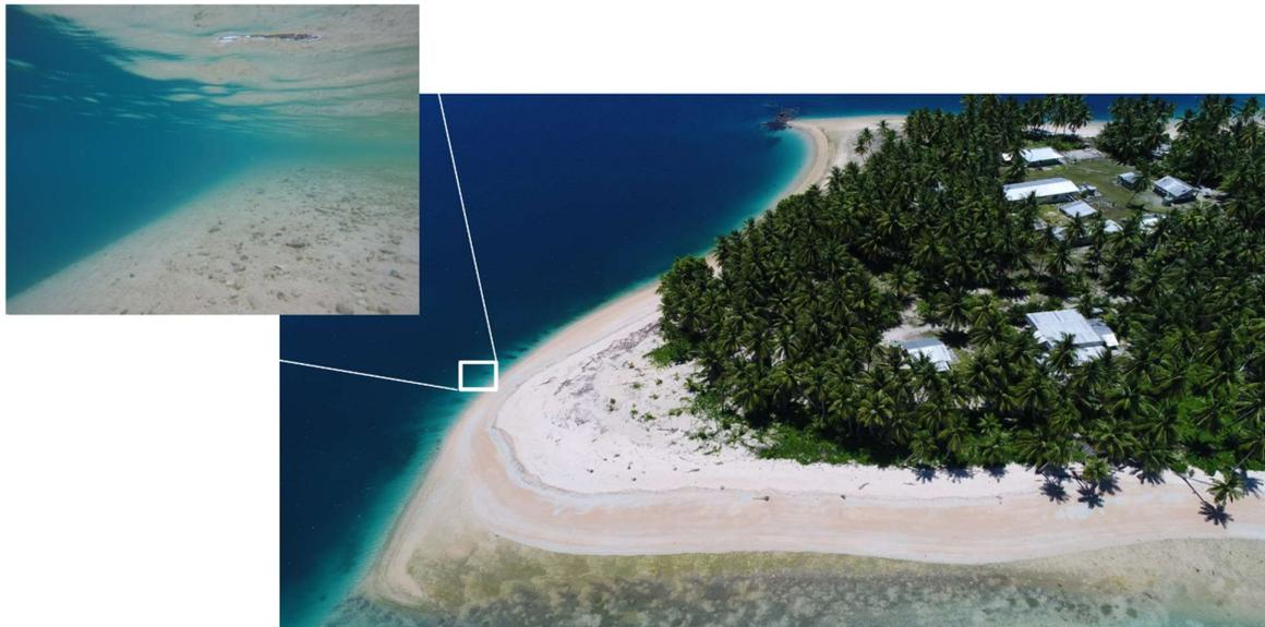
Figure 41: 'Drop overs' when sediment deposits on the north facing slope at the north-west tip of Nanumea (source imagery: SPC)
