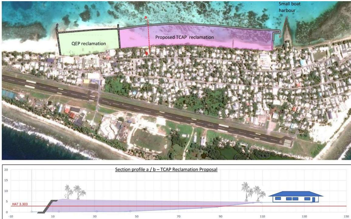
Figure 1: Proposed layout and section profile of the TCAP reclamation in Funafuti (Source: TCAP, 2019)
