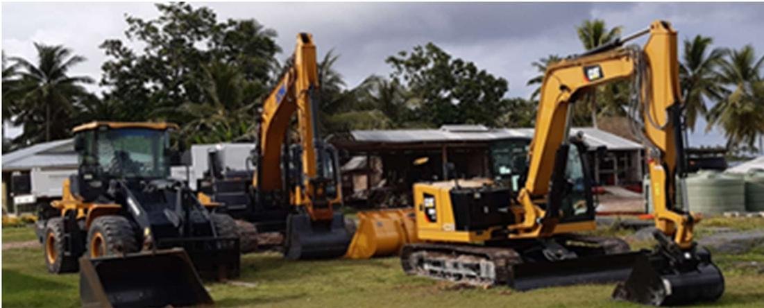
**Figure 65: Tuvalu Public Works Department (PWD) machinery on Nanumea currently undertaking upgrades to the school; Loader, 20T dump truck, 20T excavator, 8T excavator. (source: TCAP, 2020).**
