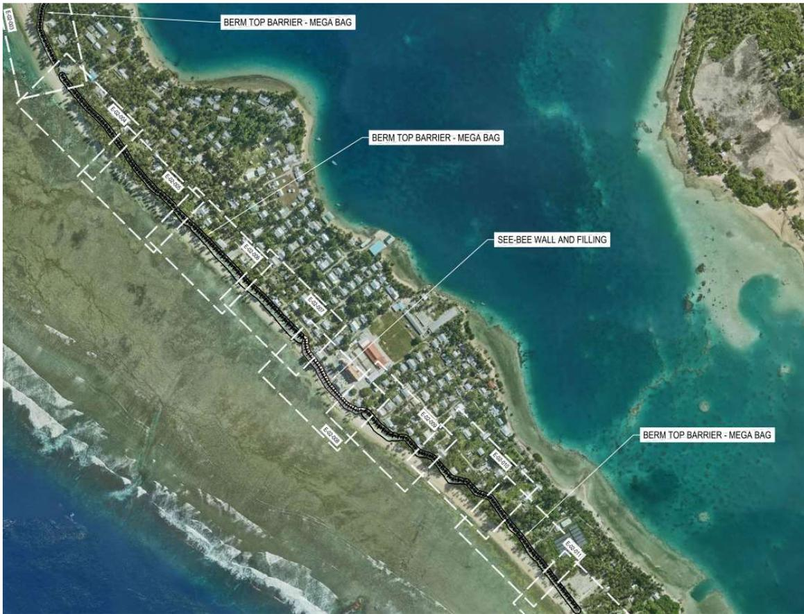
Figure 80: General alignment of the Berm top Barrier concept design and footprint on Nanumea.
