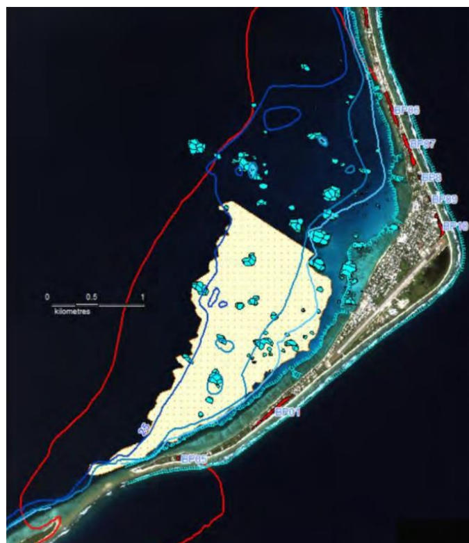
Figure 37: Impact zone expected from dredging. Red line is limit of impact area; shaded area is extraction zone examined. Light blue patches and lines are coral reefs. Blue lines are depth contours 10, 15 and 25m. Source: Hydrodynamic Model of Funafuti: Water Circulation and Applications, SOPAC Technical Report 133
