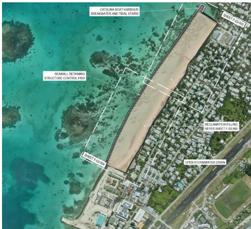
Figure 39: Proposed reclamation area and breakwater
