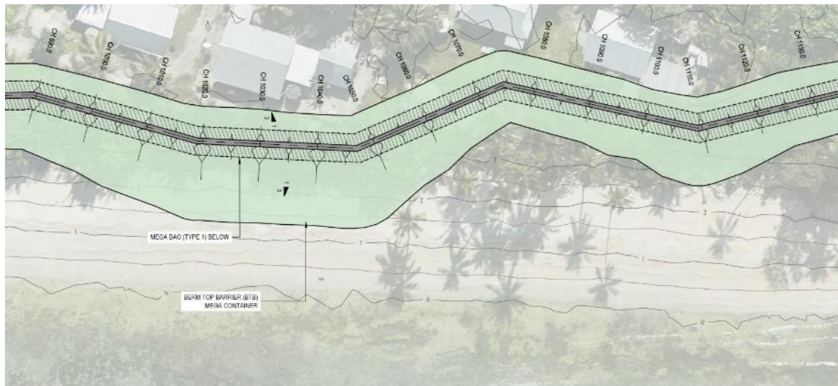
Figure 10: Example of Nanumea BTB design path avoiding buildings
