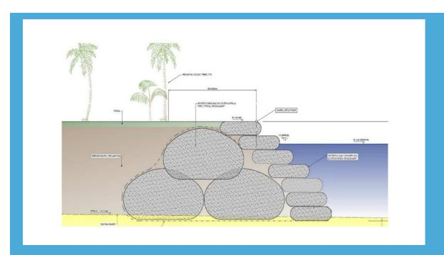
The reclamation will be filled to a height of 2m above the highest measured sea level at Funauti (highest astronomical tide (HAT). The surface will be slopped to ensure good drainage and will have a natural berm and buffer at the seaward edges to help minimum 20m constructions set back area from the landward edge of the reclamation bund.
